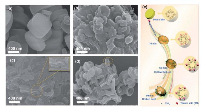
Fig. 2 SEM images of (a) NH<sub>2</sub>-MIL-125, (b) HRBC-MOF-30, (c) HRBC-MOF-60, and (d) HRBC-MOF-90. (e) Schematic illustration of the process of HRBC-MOF-x
