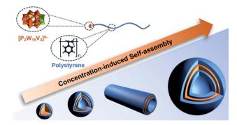
Fig. 6 The morphology evolution of concentration-induced POM-PS hybrid assembles.
