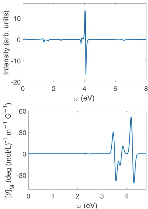
Fig. 11 Upper panel: circular dichroism spectrum eqn (9) of polaritons with  $\delta = 0$ ,  $g = 1.028 \times 10^{-1} \text{ V \AA}^{-1}$  excited by linearly polarized pulse. Lower panel: magnetic circular dichroism of Mg-porphyrin molecule in the magnetic field of 8 T (or  $3.4035 \times 10^{-5}$  a.u.).
