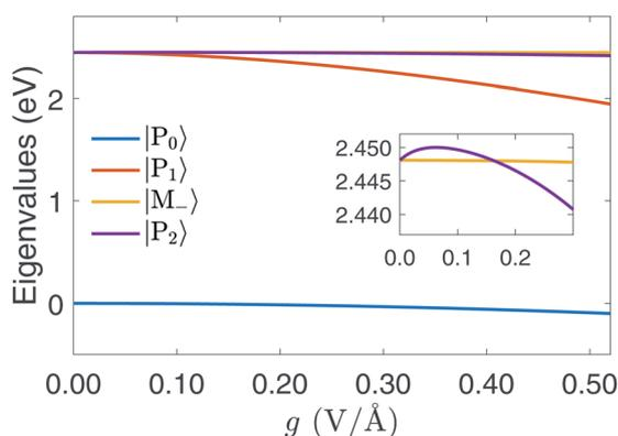
Fig. 3 Polariton energy variation with  $g$  for detuning  $\delta = 0$ . The splitting of  $|P_1\rangle$  and  $|P_2\rangle$  increase with  $g$ . The energy of  $|P_2\rangle$  is lower than  $|M_-\rangle$  for  $g > 0.16 \text{ V \AA}^{-1}$ .
