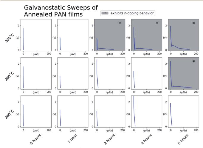
Fig. 3 Voltage profiles obtained during the 1.0 μA cm<sup>-2</sup> galvanostatic sweeps of PAN@SS electrodes annealed at each condition. The shaded backgrounds indicate that the PAN@SS electrodes annealed at those conditions undergo an n-doping reaction as demonstrated by the slight rise in voltage at potentials approaching 10 mV vs. Li/Li+ followed by a sloping voltage plateau.
