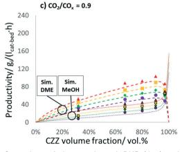
Fig. 3 Comparison of the experimental DME (dots) and MeOH (framed dots) productivities and the simulated values (dashed lines) for a CZZ volume fraction variation at 30 bar, 2.78 s<sup>-1</sup>, and 483-513 K and the three  $CO_2/CO_x$  inlet ratios of 0.6 (a), 0.75 (b) and 0.9 (c) with 20 vol% total  $CO_x$  in the feed.
