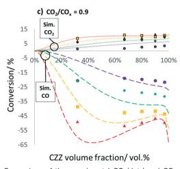
Fig. 4 Comparison of the experimental CO (dots) and CO<sub>2</sub> (framed dots) conversion and the simulated values (dashed lines) for a CZZ volume fraction variation at 30 bar, 2.78 s<sup>-1</sup>, and 483-513 K and the three  $CO_2/CO_x$  inlet ratios of 0.6 (a), 0.75 (b) and 0.9 (c) with 20 vol% total  $CO_x$  in the feed.
