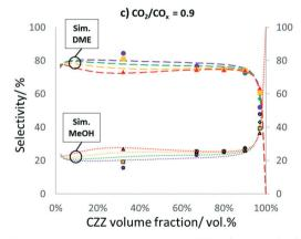
Fig. 5 Comparison of the experimental DME (dots) and MeOH (framed dots) selectivity and the simulated values (dashed lines) for a CZZ volume fraction variation at 30 bar, 2.78 s<sup>-1</sup>, and 483-513 K and the three  $CO_2/CO_x$  inlet ratios of 0.6 (a), 0.75 (b) and 0.9 (c).
