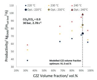
Fig. 6 Comparison of the experimental DME productivity in the run-in period and the model-optimized CZZ/FER volume ratio of 91.5/8.5 at  $CO_2/CO_x = 0.9$ , 30 bar, 2.78 s<sup>-1</sup> and three different temperatures.
