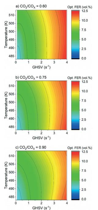
Fig. 7 Contour plots of the optimal FER volume fraction in view of maximum DME productivity under the variation of temperature and GHSV at 30 bar and CO<sub>2</sub>/CO<sub>x</sub> inlet ratios: 0.6 (a), 0.75 (b) and 0.9 (c).
