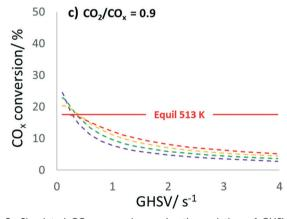
Fig. 8 Simulated CO<sub>x</sub> conversion under the variation of GHSV with the optimized CZZ/FER catalyst beds at 30 bar and 483-513 K for the CO<sub>2</sub>/CO<sub>x</sub> inlet ratios of 0.6 (a), 0.75 (b) and 0.9 (c) and the respective thermodynamic equilibrium at 513 K.
