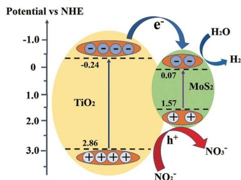
Fig. 13 Schematic illustration of the energy band structure and electron–hole separation of MoS<sub>2</sub>/TiO<sub>2</sub> composites. Reproduced from ref. 83 with permission from [Royal Society of Chemistry], copyright [2021].
