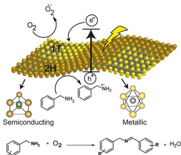
Fig. 8 Plausible mechanism for the oxidative coupling of benzylamine to imine photocatalyzed by mixed-phase 2D-MoS<sub>2</sub> nanosheets. Reproduced from ref. 77b with permission from [John Wiley & Sons, Inc.], copyright [2018].
