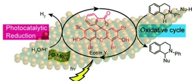
Fig. 9 Schematic illustration of the 2D-MoS<sub>2</sub> photocatalyzed oxidation and reduction cycles in presence of Eosin Y as photosensitizer. Reduction cycle produces H<sub>2</sub> from water as reported earlier, whereas oxidative cycle is responsible for CDC Reaction and formation of additional H<sub>2</sub>. Reproduced from ref. 77c with permission from [Royal Society of Chemistry], copyright [2019].
