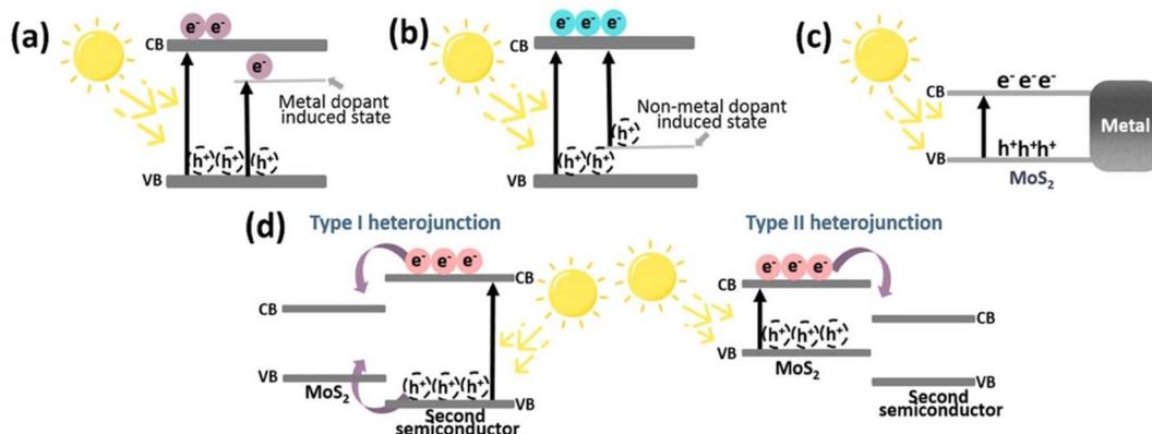
Fig. 4 Modifications of MoS<sub>2</sub> to improve its photocatalytic activity; (a) metal doping of MoS<sub>2</sub>, (b) nonmetal doping of MoS<sub>2</sub>, (c) metal deposited on MoS<sub>2</sub>, and (d) formation of a heterojunction with a second semiconductor. Reproduced from ref. 29 with permission from [American Chemical Society], copyright [2022].
