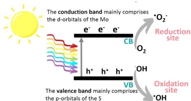
Fig. 3 Schematic illustration of the photocatalytic mechanism of MoS<sub>2</sub>. Reproduced from ref. 29 with permission from [American Chemical Society], copyright [2022].
