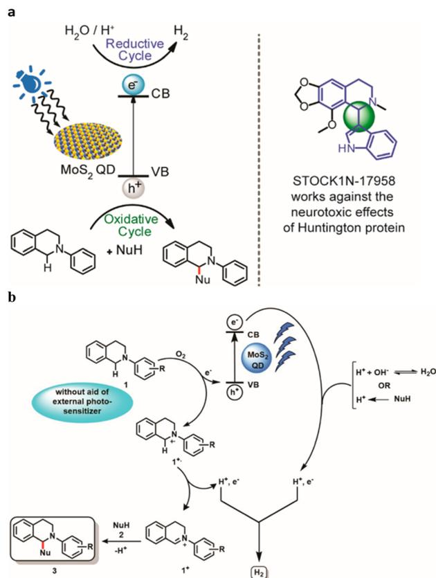
Fig. 7 (a) Photomediated oxidation and reduction cycle of MoS<sub>2</sub> QDs. (b) Proposed mechanism for the catalytic activity of MoS<sub>2</sub> blue QDs in CDC reaction synchronized with HER. Reproduced from ref. 77a with permission from [American Chemical Society], copyright [2022].
