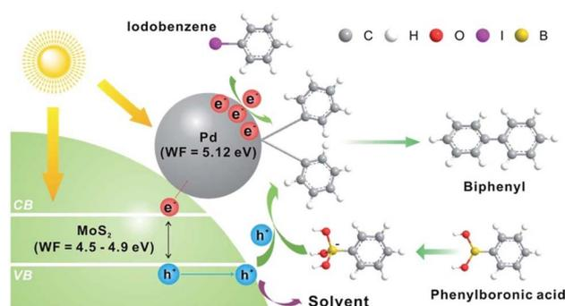
Fig. 10 The Pd-nanodot decorated MoS<sub>2</sub> micro/nanosheet for an efficient visible light induced photocatalytic Suzuki-Miyaura coupling reaction. Reproduced from ref. 78 with permission from [Royal Society of Chemistry], copyright [2017].
