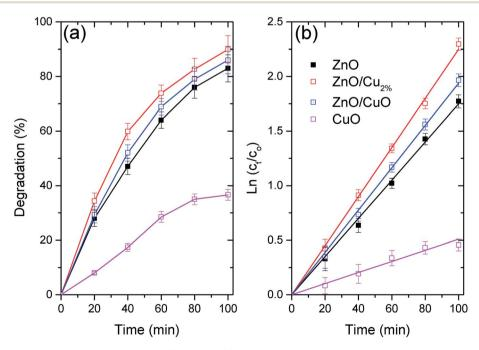
Fig. 6 Photocatalytic degradation of MO with ZnO, ZnO/Cu $_{2\%}$ , ZnO/CuO, and CuO under UV radiation. (a) Degradation percentages of MO, and (b) degradation data fitted using the first-order kinetic model.
