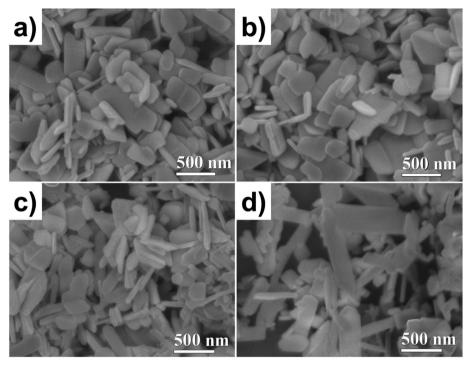
Particle morphology in SEM images for (a) ZnO, (b) ZnO/Cu<sub>2%</sub>, (c) ZnO/CuO, and (d) CuO NPs
