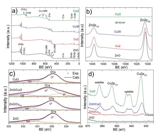
Fig. 5 XPS spectra for all samples. (a) Survey spectra and (b) Zn 2p, (c) O 1s, and (d) Cu 2p regions.
