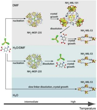
Fig. 8 Sequence of events during the crystallization of terephthalatebased MOFs in different media: low precursor concentrations (DMF); high precursor concentrations (H<sub>2</sub>O/DMF or H<sub>2</sub>O). C: grey, H: white, N: blue, O: red, Al: yellow, Cl: green. (Reprinted with permission from ref. 38. Copyright © 2011 WILEY-VCH Verlag GmbH & Co. KGaA, Weinheim.)
