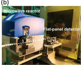
Fig. 6 Photographs of the experimental setting for in situ X-ray total scattering measurements at BL08 W (SPring-8). The photographs show the beam path through the vias (a) and the position of the vial fixed in the microwave reactor (b). Scattering data were recorded every 60 s. (Reprinted with permission from ref. 57. Copyright © 2017, American Chemical Society.)
