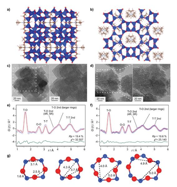
Fig. 7 Structure models of (a) MFI and (b) \*BEA. Transmission electron micrography images of (c) MFI and (d) \*BEA. Refined ex situ PDF data for (e) MFI and (f) \*BEA zeolites. Experimental data (blue circles), simulated PDF (red lines), and difference curve (green curve), (g) Typical ring structures of MFI; T-atoms: blue, O-atoms red. (Reprinted with permission from ref. 57. Copyright © 2017, American Chemical Society.)
