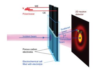
Fig. 11 Experimental setup for in situ studies of ion adsorption on the surface of microporous carbon electrodes. (Reprinted with permission from ref. 69. Copyright © 2013 WILEY-VCH Verlag GmbH & Co. KGaA, Weinheim.)
