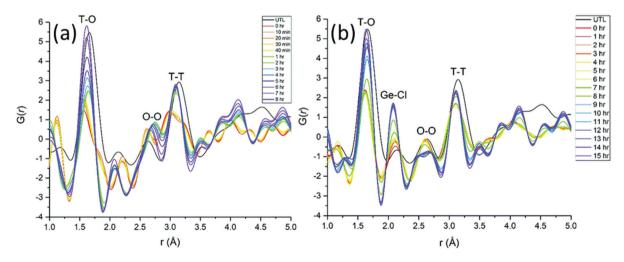
Fig. 5 Time-dependent experimental PDFs were collected (a) during 8 h of hydrolysis at 100 °C of UTL in water, (b) during rearrangement of UTL treated in 6 M HCl within 15 h at 100 °C. (Reprinted with permission from ref. 55. Copyright © 2018, The Royal Society of Chemistry.)
