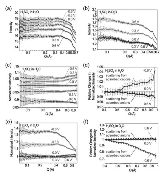
Fig. 12 In situ SANS patterns of porous carbon electrodes with (a) H<sub>2</sub>O and (b) D<sub>2</sub>O-based electrolytes during the application of a potential between the working electrode and the counter electrode. SANS profiles normalized by 0 V for (c) H2O and (d) D2O. (e) and (f) relative changes in the intensity of the normalized SANS profiles. (Reprinted with permission from ref. 69. Copyright © 2013 WILEY-VCH Verlag GmbH & Co. KGaA, Weinheim.)
