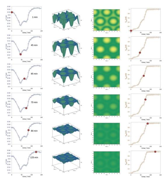
Fig. 9 Left graphs represent the change of the unit cell parameters with adsorption time, the 3D and 2D representations of the electron densities are shown in the centre, and the relative volume adsorbed is plotted in the right column. The red dots indicate unit cell parameters and  $V_{ads}$  (rel) at the respective time intervals. (Reprinted with permission from ref. 65. Copyright @ 2020 American Chemical Society.)
