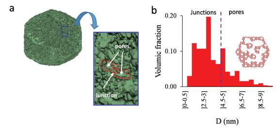
Fig. 8 (a) Tomography view of a representative crystal corresponding to the small multihollow silicalite-1 sample. The size of the sample is about  $185 \times 150 \times 115 \text{ nm}^3$ . The porosity is shown in green. (b) Cavity size distribution as seen from electron tomography.
