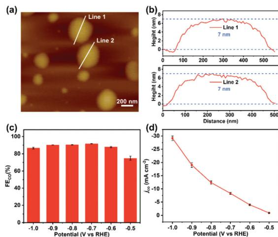
**Fig. 6** (a) The atomic force microscopy topographical image. (b) Corresponding height curves of (a). (c) FE<sub>CO</sub> of TPPDA-CoPor-COF-NSs. (d) Lasting stability test of TPPDA-CoPor-COF-NSs at -0.7 V.
