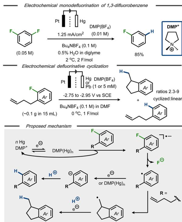
Fig. 2 Top: Selective monodefluorination of 1,3-difluorobenzene.<sup>25</sup> Middle: Defluorinative reductive cyclization.<sup>27</sup> Bottom: Mechanistic proposal for reductive hydrodefluorination.<sup>25–27</sup>
