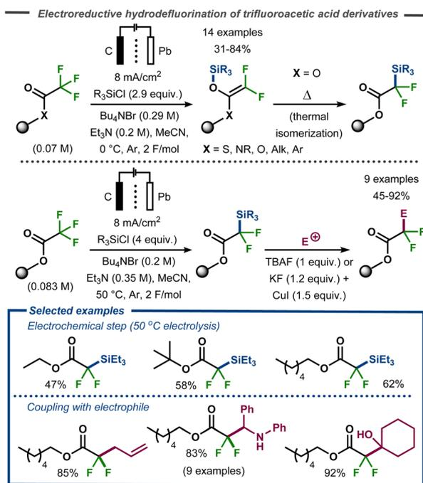
Fig. 22 Electrochemical defluorinative C–Si bond formation and subsequent functionalization.<sup>75</sup>
