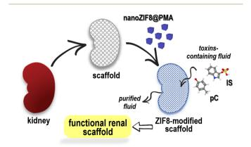
Scheme 1 Schematic illustration of the use of nanoZIF-8@PMA to modify a renal scaffold and provide it with the necessary functionality to eliminate uremic toxins, specifically p-cresol (pC) and indoxyl sulphate
