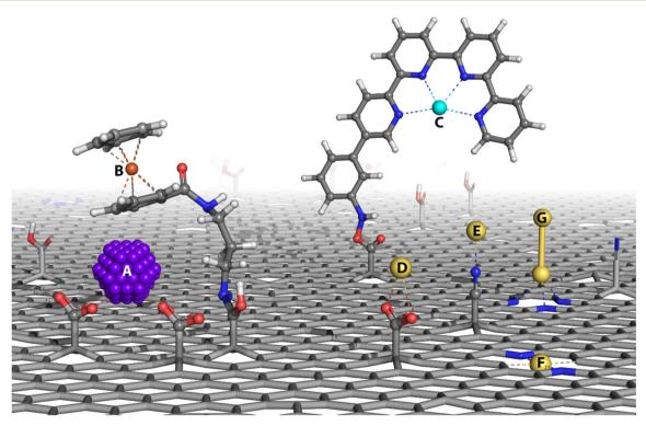
Fig. 5 A depiction of so far investigated routes to anchoring SMSs for utilization as SACs to graphene derivatives. (A) Immobilization of nanoparticles by covalently grafted functional groups. Conjugation of carboxyl groups of GA with (B) ferrocene and (C) Co quaterpyridine metal complexes. Coordination of SMS to (D) carboxyl group of GA, (E) nitrile group of GCN. Anchoring of (F) SMS and (G) metal atom dimer to defects in the structure of graphene and nitrogen-doped graphene.
