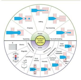
**Fig. 6** Schematic of droplet generation in passive and active methods<sup>95</sup> (this figure has been reproduced from ref. 95 with permission from Royal Society of Chemistry, copyright 2001).
