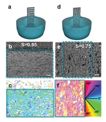
Fig. 7 Assembly in the (a) convective and (d) Landau–Levich regimes, where the (b and e) degree of disorder between assembled helices varies. (c and f) The order parameter, S, was obtained by treating the images to determine the orientation of the helices relative to the withdrawal direction. Scale bars represent 1  $\mu$ m. Reproduced with permission from ref. 102. Copyright 2020 American Chemical Society.
