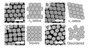
Fig. 8 The (a)  $\Lambda_0$ -lattice, (b)  $\Lambda_1$ -lattice (c) square lattice, and (d) disordered assembly patterns observed in SEM micrographs. Scale bars represent 2 μm. Reproduced with permission from ref. 95. Copyright 2019 American Chemical Society.
