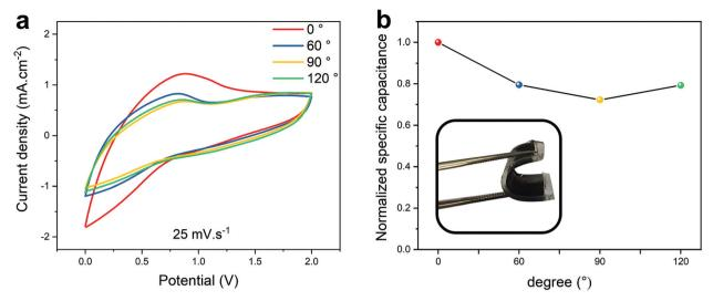
Fig. 8 Performance of the ACNTA-PANI/PDMS device under different bending angles. (a) CV curves at 25 mV s<sup>-1</sup>. (b) Normalized specific capacitance calculated from the CV curves over the bent angle. The inset illustrates the flexibility of the devices under different angles.
