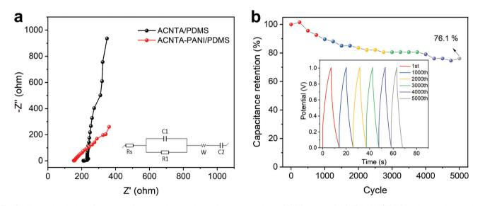
Fig. 6 Electrochemical performance of symmetric two-electrode supercapacitors. (a) EIS curve of ACNTA-PANI/PDMS at frequencies varying between 10<sup>-1</sup> and 10<sup>5</sup> Hz; the inset shows the equivalent circuit used for fitting the experimental data. (b) GCD stability of ACNTA-PANI/PDMS in a potential range between 0 and 1 V for 5000 cycles.
