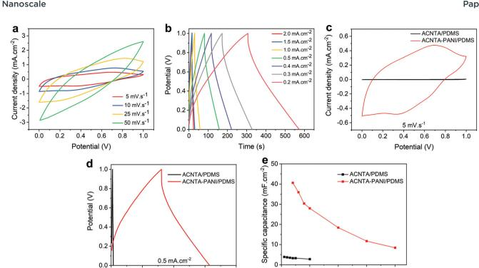
Fig. 5 Electrochemical performance of symmetric two-electrode supercapacitors. (a) CV curves of ACNTA-PANI/PDMS at scan rates varying between 5 and 50 mV s<sup>-1</sup>. (b) GCD curves at different current densities. (c) CV curves of ACNTA/PDMS and ACNTA-PANI/PDMS at a scan rate of 5 mV s<sup>-1</sup>. (d) GCD curves of ACNTA/PDMS and ACNTA-PANI/PDMS at 0.5 mA cm<sup>-2</sup>. (e) Areal specific capacitances calculated for different current densities.
