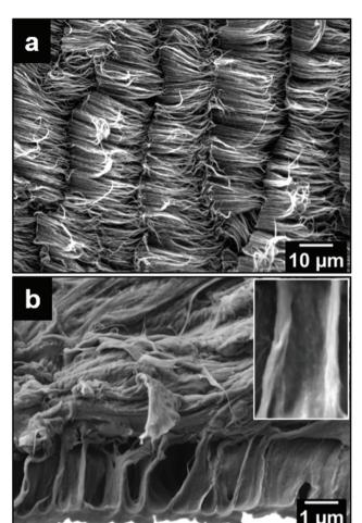
**Fig. 2** (a) Top-view SEM image of the horizontally aligned carbon nanotubes (HA-CNTs) that were bent during the wafer drop casting process. (b) Cross-sectional SEM image of the flexible electrode showing HA-CNTs on top of vertically aligned carbon nanotubes (VA-CNTs) densified when in contact with the polydimethylsiloxane (PDMS) matrix. PANI is a thin indistinguishable layer spread across the HA-CNTs/air interface.
