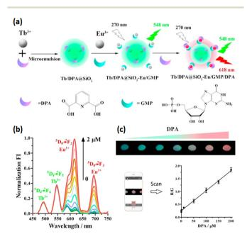
Fig. 10 Anthrax biomarker (DPA) detection via a dual-lanthanide based silica NPs. (a) Representation of the luminescent probe. (b) Emission spectra of Tb/DPA@SiO2-Eu/GMP probe to different concentrations of DPA upon DPA excitation. (c) Fluorescence color image of the designed paper-based visual sensor over various concentrations of DPA solution under 254 nm UV light excitation and standard curve obtained with a smartphone. Reprinted from ref. 188, Copyright (2017), with permission
