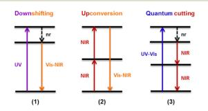
Fig. 1 Schematic representation of different spectral conversion mechanisms possible with  $Ln^{3+}$ -doped NPs. nr = non-radiative.
