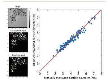
Fig. 3 The left panel shows the TEM image, ground truth mask, and predicted mask. The right panel compares the manually measured particle diameter with the deep learning-based computed particle diameter.
