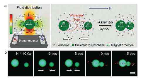
Fig. 43 Ferrofluid-driven assembly of dielectric microspheres: (a) schematic illustration of the field distribution around a polystyrene (PS) microsphere on top of a planar magnet (left) and the potential trap of magnetostatic forces between microspheres dispersed in a ferrofluid. (b) Optical microscopy images of a pair of PS microspheres in a ferrofluid under a magnetic field of 40 Gs. Scale bar is 10 μm (reproduced from ref. 709 with permission from John Wiley and Sons, copyright 2021).
