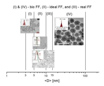
Fig. 2 Particle size ranges for ferrofluids and bio-ferrofluids: (I) bio-ferrofluids (2–5 nm) (reproduced from ref. 47 with permission from MDPI, copyright 2020), (II) ideal ferrofluids (5–10 nm), (III) conventional (real) ferrofluids (5–15 nm), and (IV) bio-ferrofluids (15–100 nm) (reproduced from ref. 44 with permission from *Am. Chem. Soc.*, copyright 2020).
