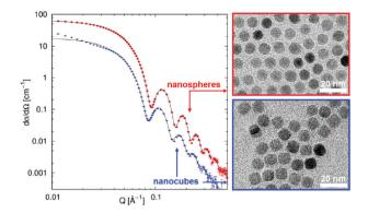
Fig. 15 SAXS curves from diluted solutions of oleic acid-capped maghemite nanospheres and nanocubes in toluene combined with TEM image from dried samples (reproduced from ref. 314 with permission from IOP Publishing - Open Access, copyright 2012).
