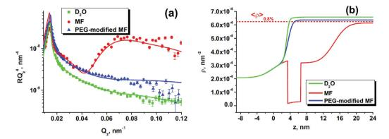
Fig. 21 (a) Experimental reflectivity curves (Fresnel representation) together with fits (solid lines) for pure D<sub>2</sub>O (green squares), initial aqueous MF (red circles) and PEG-modified MF (blue triangles); (b) found from experimental data SLD profiles for three studied kinds of solid/liquid interfaces. The calculated mean SLD for the initial ferrofluid (concentration 0.8%) is shown (dashed line) for comparison (reproduced from ref. 366 with permission from Elsevier, copyright 2017).
