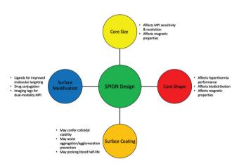
Fig. 3 Important structural modifications that could be considered when synthesising a SPION tailored for different MPI applications.
