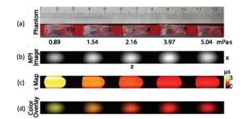
Fig. 27 Multi-colour MPI images for viscosity mapping. (a) An imaging phantom of 5 different samples of SPIONs in increasing viscosity levels from 0.89 mPa s to 5.04 mPa s. (b) The MPI images for each sample, with (c) their corresponding relaxation ( $\tau$ ) maps. (d) The color overlay between the  $\tau$  maps and MPI images for each sample. Reproduced with permission of IOP Publishing, from ref. 22; permission conveyed through Copyright Clearance Center, Inc.
