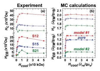
Fig. 11 (a) Experimentally determined exchange bias ( $H_{EB}$ , full circles) and coercive fields ( $H_C$ , half-full circles) and (b) Monte Carlo calculations of  $H_{EB}$  (full triangles) and  $H_C$  (half-full triangles) for the three heterostructured nanocrystal models (Fig. 1).
