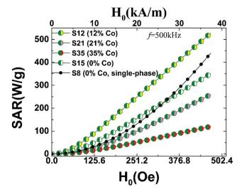
Fig. 12 Specific absorption rate (SAR) calculated on the grounds of susceptibility losses (AC field amplitude,  $H_0$  and f = 500 kHz) for Co-substituted heterostructured nanocrystals (15 nm), which are compared with 8 nm (S8) and 15 nm (S15) Fe-containing only<sup>34</sup> nanocrystals; SAR values are derived in view of the linear response theory of a modified Néel-Brown relaxation Monte Carlo model.
