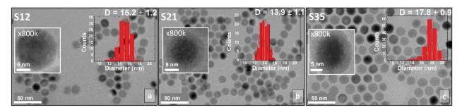
Fig. 3 Low-magnification bright-field transmission electron microscopy (TEM) images of core@shell  $Co_x Fe_{1-x} O@Co_y Fe_{3-y} O_4$  spherical nanocrystals and insets of high-resolution TEM images of selected particles at 800k magnification. The nanoparticle size distributions are also shown as insets.
