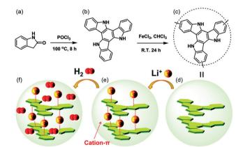
(a)-(c) Synthetic route for the conjugated microporous polymer PTAT. Schematic representation showing the installation of lithium-doped CMP Li<sup>+</sup>-PTAT through point-to-face cation- $\pi$  interactions (d and e) and its hydrogen adsorption (f). Reproduced from L. Yang, Y. Ma, Y. Xu, G. Chang, Chem. Commun., 2019, 55, 11227-11230 with permission from The Royal Society of Chemistry.
