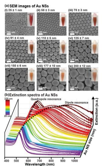
Fig. 1 Qualitative analysis of the relationships between Au nanospheres (NSs) size, size distribution, and LSPR. (a) SEM images of Au NSs with different sizes. Corresponding digital images of the Au NS dispersions are shown in the insets. (b) Extinction spectra of the Au NSs of different sizes.
