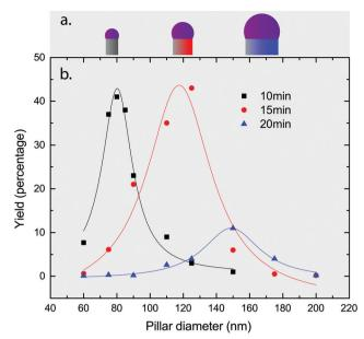
Fig. 3 (a) Schematics showing the increase in droplet volume with SiO<sub>2</sub>/Si pillar diameter at a fixed contact angle. (b) Vertical yield as a function of SiO<sub>2</sub>/Si pillar nominal diameter for Ga predeposition times of 10 min, 15 min and 20 min
