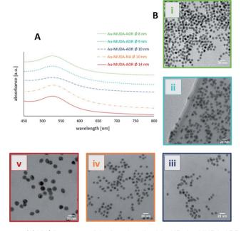
Fig. 4 (A) UV/Vis spectra of the functionalised Au NPs Au-MUDA-ADR Ø 14 nm, Ø 10 nm, Ø 9 nm, Ø 8 nm and Au-MUDA-NA Ø 10 nm with their measured absorption maxima, and (B) their corresponding TEM images of (i) Au-MUDA-ADR  $d=8.1\pm0.6$  nm, (iii) Au-MUDA-ADR  $d=8.9\pm0.8$  nm, (iii) Au-MUDA-ADR  $d=9.9\pm0.8$  nm, (iv) Au-MUDA-NA  $d=9.9\pm0.8$  nm and (v) Au-MUDA-ADR  $d=13.9\pm1.2$  nm.
