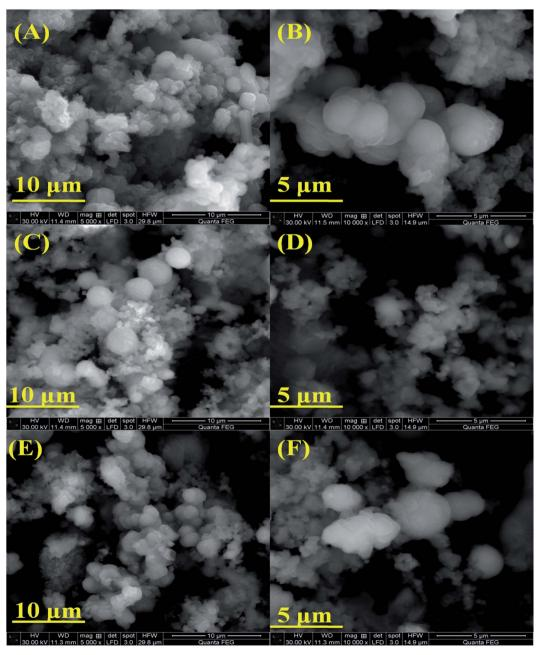
Fig. 2 SEM images (A and B) pristine NiMnO<sub>3</sub>, (C and D) 0.01 M Sm-doped NiMnO<sub>3</sub>, and (E and F) 0.02 M Sm-doped NiMnO<sub>3</sub> at 10 and 5 µm.
