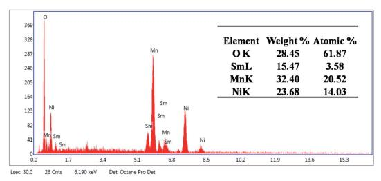
Fig. 3 An EDX spectra of 0.02 M Sm-doped NiMnO<sub>3</sub>
