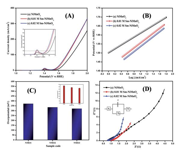
Fig. 5 (A) LSV spectra, (B) Tafel slope (C) Bar diagram (inset: error bar), and (D) EIS spectra of pristine NiMnO<sub>3</sub>, 0.01 M Sm-doped NiMnO<sub>3</sub>, and 0.02 M Sm-doped NiMnO<sub>3</sub>.
