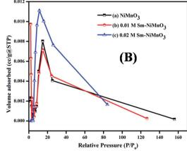
Fig. 4 (A) Nitrogen adsorption—desorption and (B) BJH pore diameter of pristine NiMnO $_3$ , 0.01 M Sm-doped NiMnO $_3$ , and 0.02 M Sm-doped NiMnO $_3$ .
