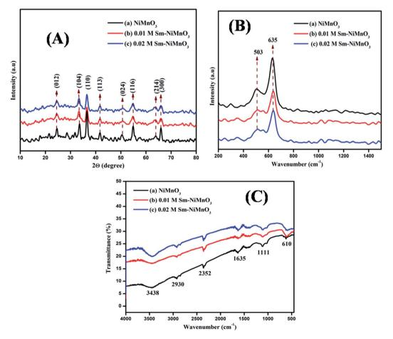
Fig. 1 (A) XRD spectra (B) Raman, and (C) FTIR spectra of pristine NiMnO<sub>3</sub>, 0.01 M Sm-doped NiMnO<sub>3</sub>, and 0.02 M Sm-doped NiMnO<sub>5</sub>.
