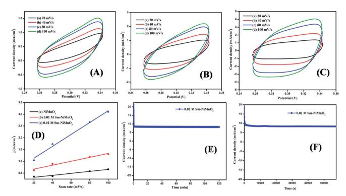
Fig. 6 (A–C) CV Curves and (D) double-layer capacitance for pristine NiMnO $_3$ , 0.01 M, 0.02 M Sm-doped NiMnO $_3$ , chronoamperometry test of 0.02 M Sm-doped NiMnO $_3$  for (E) 2 h and (F) 16 h.
