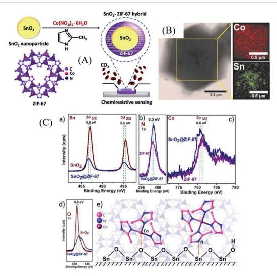
Fig. 9 (A) Schematic illustration of SnO<sub>2</sub>@ZIF-67 architecture formation, (B) TEM image of the core-shell SnO<sub>2</sub>@ZIF-67 material with its corresponding EDX-elemental analysis, and (C) XPS analysis to examine the synergistic effect of SnO2 and the ZIIF-67 MOF. Reproduced from ref. 101 with permission from Wiley-VCH GmbH, copyright 2021.
