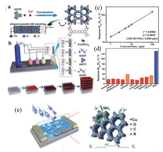
Fig. 3 (a) Illustration of the crystal structure of Cu<sub>3</sub>(HHTP)<sub>2</sub>. (b) Fabrication of the Cu<sub>3</sub>(HHTP)<sub>2</sub> thin film by a spray layer-by-layer (LBL) method using the LPE technique, (c) LOD graph, (d) selectivity test of the  $Cu_3(HHTP)_2$  thin-film sensor, and (e)  $NH_3$  sensing mechanism of the  $Cu_3(HHTP)_2$ thin film sensor at RT. Reproduced from ref. 70 with permission from Wiley Sons, copyright 2021.
