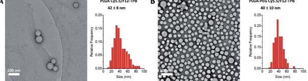
Fig. 2 TEM images (left) and corresponding size distribution histograms (right) for PLGA (A) and PLGA-PEG (B) NPs loaded with 20 mM Cy5.5/ F12-TPB dye. The values correspond to the average NP diameter, while errors correspond to the half-width at the half maximum. At least 200 NPs were analyzed per condition.
