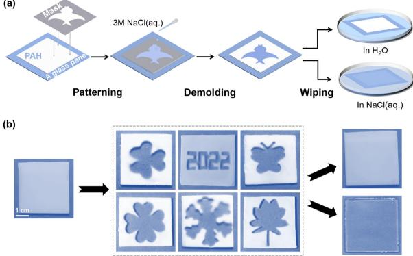
(a) Schematic demonstration of patterning on the gel through NaCl(aq.) painting. (b) Images of different painted patterns on PAH, the scale bar is Fia. 3 1 cm.
