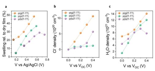
**Fig. 3** (a) Polymer swelling relative to the corresponding dry state. Star symbols correspond to the swelling values of the film at  $V_{OC}$  conditions (*i.e.*, passive swelling). The voltage values are plotted vs. Ag/AgCl. (b) Chloride ion and (c) water molecule density in the conjugated polymer film following electrochemical doping at various potentials against  $V_{OC}$ .  $V_{OC}$  values are 0.14 V for p(g2T-TT), 0.19 V for p(p2T-TT), and 0.35 V for p(b2T-TT).
