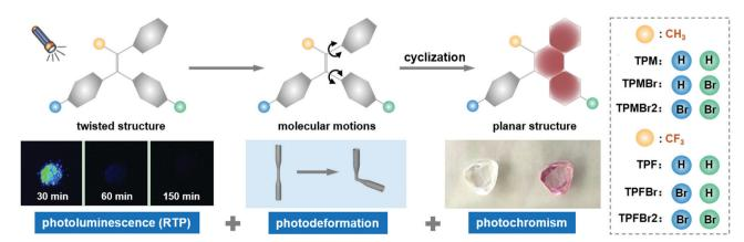
Fig. 1 Chemical structures and photoinduced cyclization process of triphenylethylene derivatives as well as schematic diagram of multiphotoresponsive properties.
