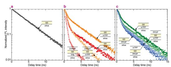
Fig. 4 Time-resolved photoluminescence decay. Mesolight<sup>®</sup> blue-QDs (20 nm thick film): (a) on fused silica, (b) on the polymer HTL, before and after deposition of ZnMgO nanoparticles, (c) on the polymer HTL or ETL, before and after the lay down of the opposite transport layer. The fast component comes primarily from the polymer ( $\tau \approx 0.7$  ns) and the slow component from the QDs ( $\tau \approx 4.3$  ns in pristine film). Excitation, 374 nm; emission, 465 nm.
