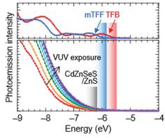
**Fig. 2** Ultraviolet photoemission spectroscopy of the ionization edge of Mesolight<sup>®</sup> blue-emitting CdZnSeS/ZnS QDs, and possible hole transporting organic semiconductors. Excitation source, He–I. Energy plotted from the vacuum level. He–I radiation causes dehydrogenation of the unsaturated organic acid coating, which reveals the VB onset at *ca.* –6.2 eV. The effective VB edges of TFB and mTFF are –5.5 and –5.8 eV, respectively, extrapolated from inflection of the frontier slope.
