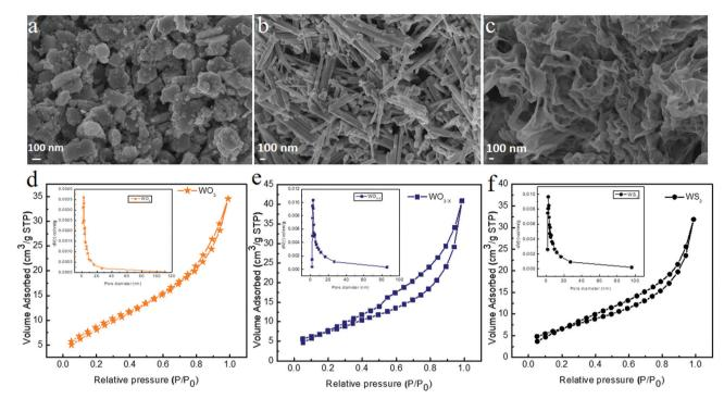
Fig. 4 FESEM images of (a) WO<sub>3</sub>, (b) WO<sub>3-x</sub> and (c) WS<sub>2</sub>, and nitrogen adsorption and desorption isotherms of (d) WO<sub>3</sub>, (e) WO<sub>3-x</sub> and (f) WS<sub>2</sub>
