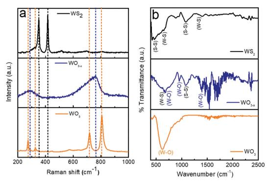
Fig. 3 (a) Raman spectra, and (b) FTIR spectra of the  $WO_3$ ,  $WO_{3-x}$  and  $WS_2$  samples.
