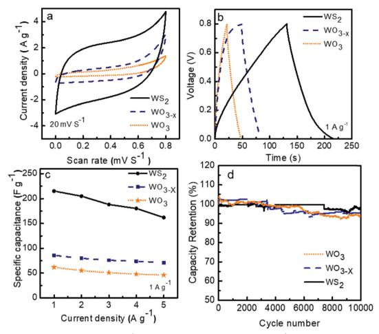
Fig. 6 (a) CV curve of  $WO_3$ ,  $WO_{3-x}$  and  $WS_2$  at 20 mV s<sup>-1</sup>, (b) GCD curve of  $WO_3$ ,  $WO_{3-x}$  and  $WS_2$  at 1 A g<sup>-1</sup>, (c) variation of the specific capacitance with current density, (d) the capacitance retention of the  $WO_3$ ,  $WO_{3-x}$  and  $WS_2$  electrode material over 10 000 cycles.
