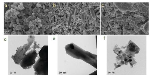
Fig. 7 SEM images of (a)  $WO_{3-x}$  (b)  $WO_{3-x}$  and (c)  $WS_2$  and TEM images of (d)  $WO_{3-x}$ , (e)  $WO_{3-x}$ , and (f)  $WS_2$  after the cycling stability test.
