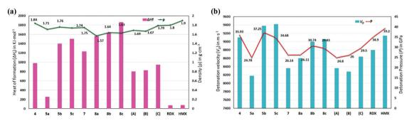
Fig. 8 Calculated heats of formation, experimental densities (a), calculated detonation velocities, and detonation pressures (b) of 4, 5a-c, 7, 8a-c, and compared with those of A, B, C, RDX, and HMX
