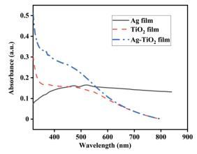
Fig. 2 Normalised absorption spectra for Aq, TiO<sub>2</sub> and Aq-TiO<sub>2</sub> SERS film.
