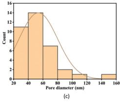
Fig. 1 Field emission scanning electron microscope (FESEM) images reveal the morphology of (a) TiO2 film with unique nanocage structure, (b) Ag coated TiO2 film, and (c) indicates the Histogram plot of pore diameters present within Ag-TiO2 nanocage film.
