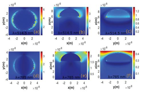
Fig. 5 Electric field distribution map at various planes for two different excitation lasers of 514.5 nm and 785 nm wavelengths respectively. (a–c) represent the field variation at XY, XZ and YZ plane for 514.5 nm, (d–f) denote the field variation at XY, XZ, and YZ planes for 785 nm excitation laser wavelength. The colour bar indicates  $\left|\frac{E_{\text{local}}}{E_{\text{incident}}}\right|$ .
