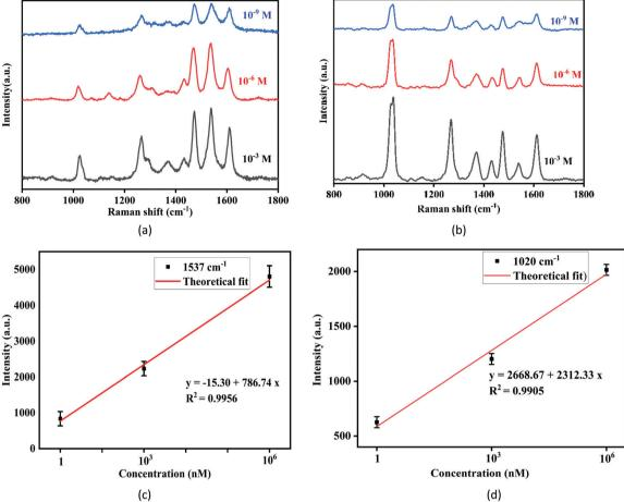
Fig. 4 SERS spectra of N719 at various concentrations from  $10^{-3}$  M to  $10^{-9}$  M on the Ag-TiO<sub>2</sub> SERS film for (a) 514.5 nm and (b) 785 nm excitation laser, and (c and d) represent their corresponding plot of SERS intensity vs. analyte concentration at 1537 cm<sup>-1</sup>, and 1020 cm<sup>-1</sup>, respectively.
