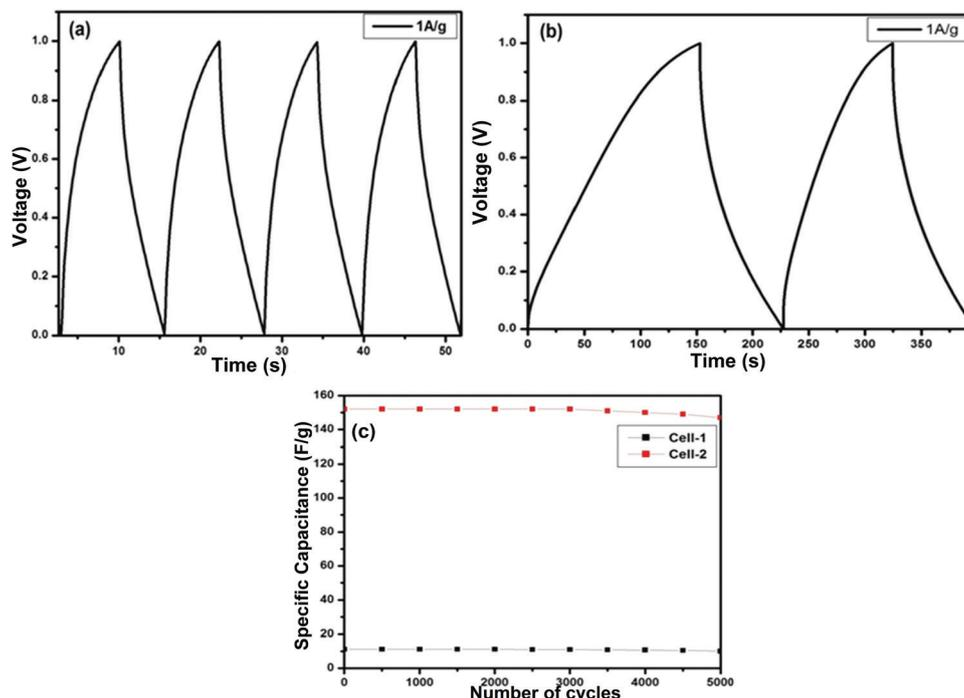
Fig. 12 GCD curves of Cell-1 and Cell-2: (a) ZGN-based cell and (b) MGN-based cell. (C) Charge–discharge over 5000 cycles for Cell-1 and Cell-2 at a current density of  $1 \text{ A g}^{-1}$  in aqueous  $1 \text{ M H}_3\text{PO}_4$  electrolyte.
