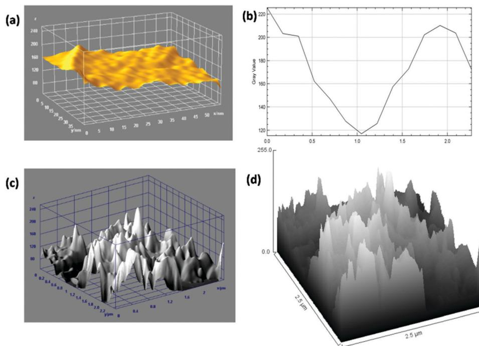
Fig. 5 (a) 3D surface plot from TEM analysis of MGNs. (b) Plot profile diagram from the thickness measurement of MGNs. (c) 3D surface topology from the SEM analysis of MGNs. (d) Hill stack plot of MGNs showing surface roughness.
