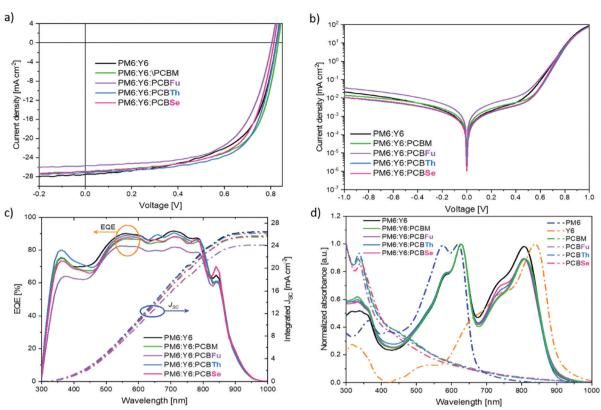
Fig. 2 Best current-density vs. voltage (J-V) characteristics under (a) simulated AM 1.5 G illumination and (b) dark conditions, and (c) EQE spectra (solid lines) and integrated J<sub>SC</sub> (dash dot lines) of binary OSCs and ternary OSCs with PCBM, PCBFu, PCBTh, and PCBSe. (d) Absorption spectra of neat PM6, Y6 and PCBM-derivatives (dash dot lines) and the blends, PM6:Y6:PCBM-derivatives (solid lines).
