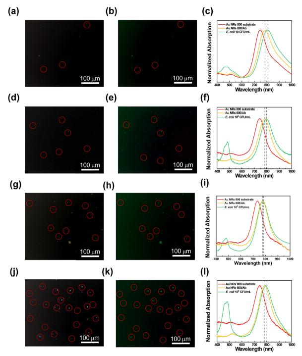
Fig. 6 Characterization of the bioactive plasmonic substrates after incubating E. coli dispersions in minimum E at different cell concentrations. Contrast phase microscopy images (a, d, g and j), fluorescence microscopy images (b, e, h and k), and absorption spectroscopy characterization (c, f, i and l) of the bioactive plasmonic substrate progressively incubated in a 10,  $10^2$ ,  $10^3$ , and  $10^4$  CFU mL<sup>-1</sup> E. coli cell dispersion.
