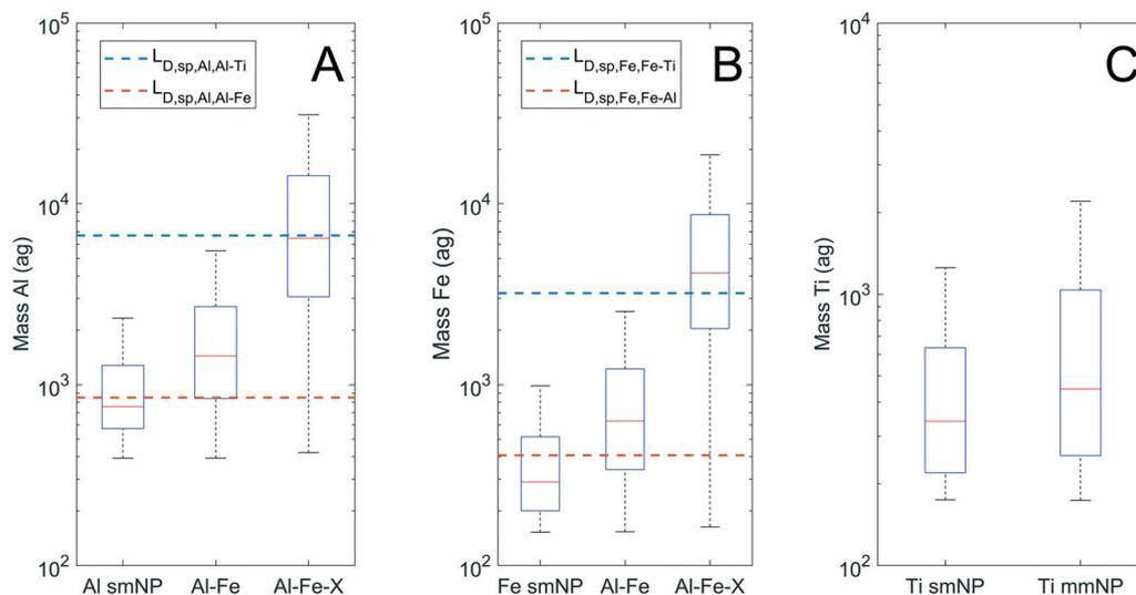
**Fig. 5** Al (A), Fe (B), and Ti (C) particle mass distributions in single metal nanoparticle (smNP) and multi metal nanoparticle (mmNP) groups. In Al-Fe-X particles, X refers to additional elements (Mg and Ti). Red lines represent the median mass, boxes represent the interquartile range (25–75%), and whiskers represent 1.5× the interquartile range. Dotted lines represent the required mass of one element to detect another element based on the crustal ratio ( $L_{D,sp,i,ij}$ ).
