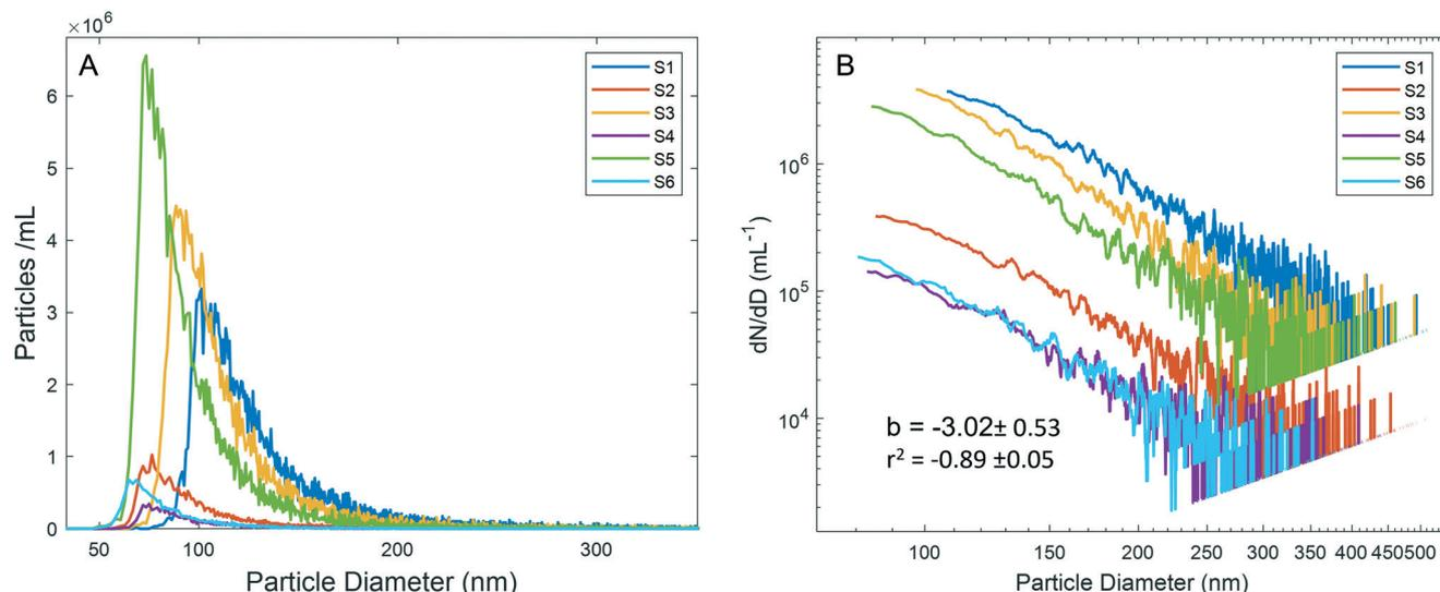
**Fig. 2** A) Particle size distributions for  $^{27}\text{Al}$  obtained by spICP-QMS. B) Reprocessed PSD data, with data normalized to number per nm ( $dN/dD$ ) versus diameter and plotted in log space. The slope ( $b$ ) and  $r^2$  are an average of all samples;  $\pm 1$  SD.
