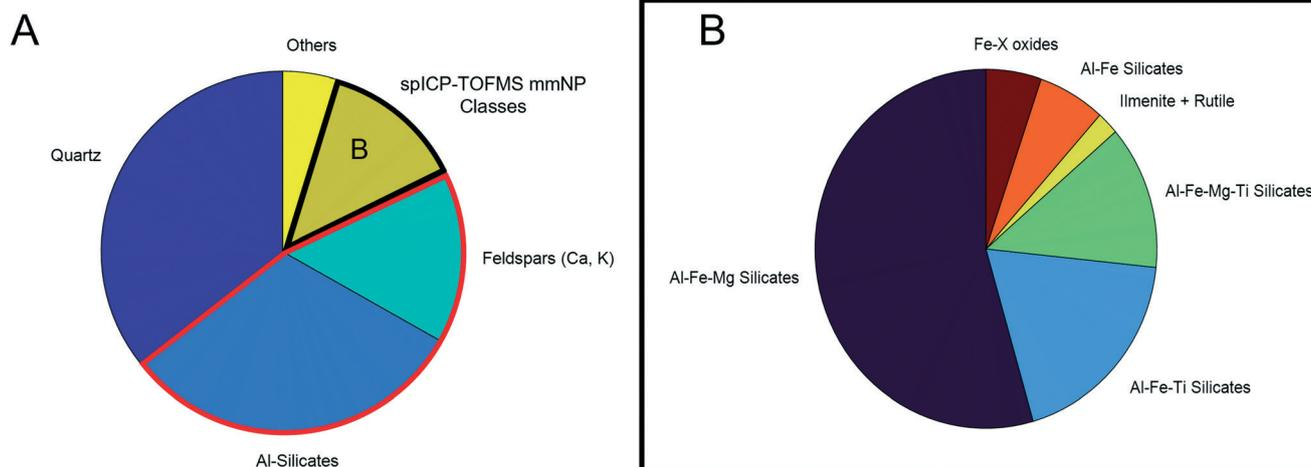
**Fig. 6** A) Mass percent of particle types/minerals detected in sample S1 by automated mineralogy (AM). The red outlined section indicates particle types that would have likely been detected as Al single metal particles (smNPs) by spICP-TOFMS due to the inability to accurately quantify the other constituents (Si, Ca, K, and Na). B) Mass percent of mineral types that overlapped in elemental composition with multi metal nanoparticle (mmNP) groups observed by spICP-TOFMS.
