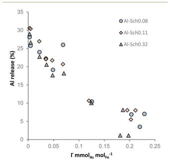
Fig. 4 Al released from Al-Sch after 72 h equilibration with the arsenate solution as a function of the adsorbed aqueous arsenate  $\left(\text{mmol}_{\text{ASO}_4} \text{ mol}_{\text{Fe}}^{-1}\right)$ .
