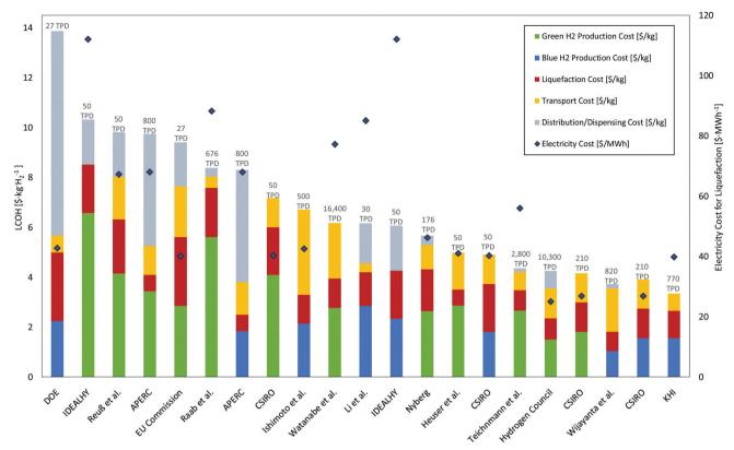
Levelised cost of hydrogen (LCOH) for proposed liquid hydrogen value chains found in literature
