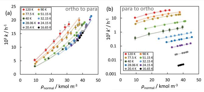
Fig. 3 Autocatalytic homogenous ortho-to-para (a) & para-to-ortho (b) conversion rate constants as a function of normal hydrogen molar density systems. The dashed curves correspond to values calculated with the empirical correlation shown in eqn (5) and (6).
