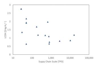
Fig. 18 Liquefaction cost component of the LCOH studies shown in Fig. 17 as a function of the supply chain scale.
