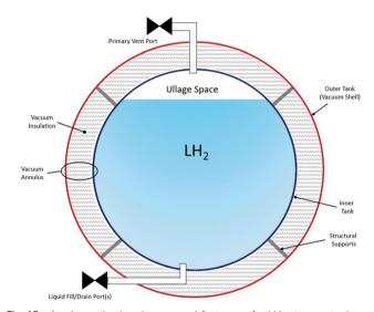
A schematic showing general features of a LH<sub>2</sub> storage tank.
