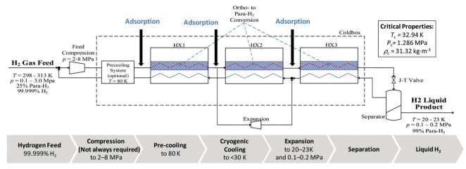
Fig. 4 Simplified schematic diagram of the hydrogen liquefaction process based on simple Claude cycle. Critical properties of para-hydrogen are shown in this schematic
