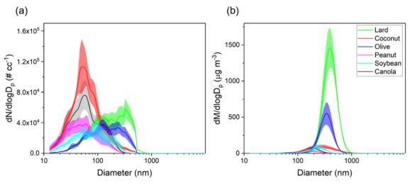
Fig. 3 Aerosol size distributions in terms of number and mass concentrations for different oils heated at 180  $^{\circ}$ C are shown in panels (a) and (b), respectively. The lines represent average values, and the shaded region represents standard error (n = 4). The particle mass distributions for lard, coconut oil, and olive oil were merged between the SMPS and APS measurements using the TSI DataMerge software.
