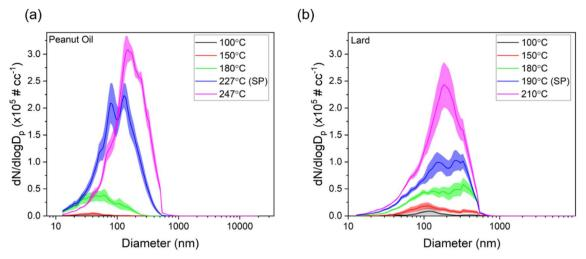
Fig. 4 Aerosol number size distributions for peanut oil and lard over different cooking temperatures are shown in panels (a) and (b), respectively. The lines represent average values, and the shaded region represents standard error (n = 4)
