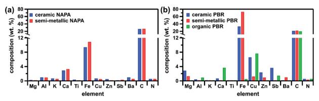
Fig. 2 Elemental composition of brake pads from (a) NAPA and (b) PBR as determined by ICP-MS and total C/total N combustion analysis. All data shown here are presented numerically in Table S4.†
