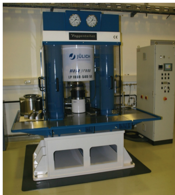
Fig. 2 The Voggenreiter LP 1000-540/50 HP/HT apparatus present in the laboratories of the Institute of Reactor Safety and Nuclear Waste Management (IEK-6), Forschungszentrum Jülich, Germany.
