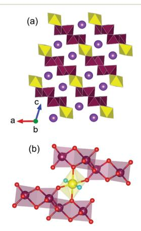
Fig. 10 (a) Structural layer motif of  $K_2[UO_2(Mo_2O_7)_2]$  highlighting the occurrence of (b) the (Mo<sub>2</sub>O<sub>7</sub>)<sup>2-</sup> unit. Note maroon and yellow polyhedra respectively represent Mo and U polyhedra whereas purple, maroon, yellow, red and agua spheres respectively represent K, Mo, U, O and uranyl-O atoms respectively. Figure adapted from ref. 67.
