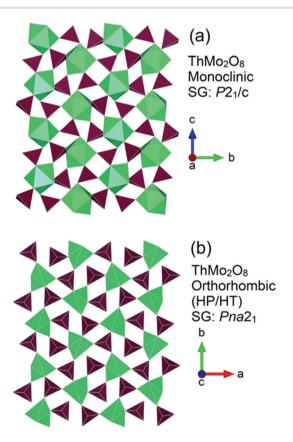
Fig. 3 General structure representations of the ThMo<sub>2</sub>O<sub>8</sub> polymorphs of (a) the ambient pressure high temperature synthesised monoclinic (SG P2<sub>1</sub>/c) and (b) the HP/HT orthorhombic (SG Pna2<sub>1</sub>). Note Th and Mo polyhedra are represented by green and maroon polygons respectively. Figure adapted from ref. 49.
