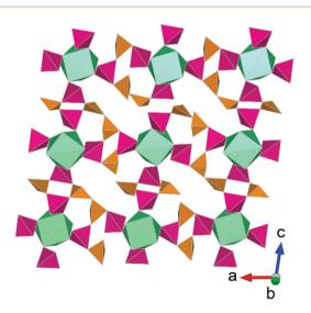
Fig. 6 Structural representation of Th(As(III)<sub>4</sub>As(v)<sub>4</sub>O<sub>18</sub>) highlighting coordination motif of different As valences in the layer plane. Note that Th polyhedra (green) are coordinated firstly by As(III)O<sub>4</sub> (orange) forming discrete clusters that are linked by As(v)O<sub>3</sub> polyhedra (pink). Figure adapted from ref. 54.
