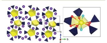
Fig. 12 Structure of Na<sub>4</sub>[(UO<sub>2</sub>)(SO<sub>4</sub>)<sub>3</sub>] synthesised from HP/HT conditions illustrating bending of the uranyl group in the inset. Note Yellow and dark polyhedra represent U and S polyhedra respectively whereas purple, yellow, red and aqua blue spheres represent K, U, O and uranyl O atoms respectively. Figure adapted from ref. 84.
