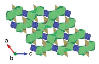
Fig. 5 Structural representation of  $Th_2Te_3O_{11}$  highlighting coordination motif of different Te valences adapted from ref. 51. Note: Th(v), Te(v) and Te(v) polyhedra are presented as green, tan and blue polygons.
