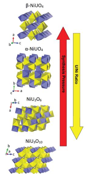
Fig. 8 Structural representations of mono-, di- and triuranates of the Ni-U-O system emphasising the relationship between the structure type and synthesis conditions. Note uranium and nickel polyhedra are given in yellow and purple respectively. Structures and conditions adapted from ref. 12.
