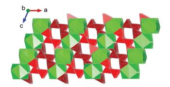
Fig. 7 Structural representation of the monoclinic channel structure of  $AnB_4O_8$  (An = Th, U), (Th variant depicted). Note Th and B polyhedra are represented by green and red polygons respectively. Figure adapted from ref. 37.
