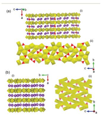
Fig. 11 Structural representations of (a) orthorhombic  $K_{12}[(UO_2)_{19}(UO_4)]$  $(B_2O_5)_2(BO_3)_6(BO_2OH)O_{10}] \cdot nH_2O$  in (i) general and (ii) layer format, and (b) monoclinic  $K_4[(UO_2)_5(BO_3)_2O_4] \cdot H_2O$  in (i) general and (ii) layer formats. Yellow and red polyhedra represent U and B polyhedra respectively whereas purple spheres represent K atoms. Figures adapted from ref. 79.
