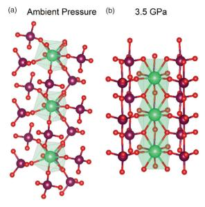
Fig. 4 Comparison of the coordination motifs between the Th and Mo polyhedra at (a) ambient pressure synthesised monoclinic variant and (b) HP/HT orthorhombic variant of  $ThMo_2O_8$ . The figure illustrates the reduced distance between Th polyhedra between the ambient and higher-pressure variants. Note Th polyhedra, Mo and O atoms are represented by green polygons, maroon and red spheres respectively. Figure adapted from ref. 49.
