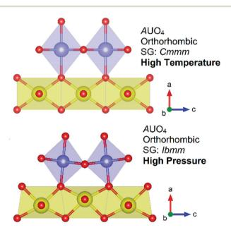
Fig. 9 Structural representations of the AUO<sub>4</sub> orthorhombic structures in space groups Cmmm and Ibmm where it has been shown high temperatures favour the Cmmm structure non-distorted structure and high pressures favour the distorted *lbmm* structure. Note the tilt in the AO<sub>6</sub> polyhedra (purple) and distortion of UO<sub>6</sub> polyhedra (yellow) w.r.t. oxygen atoms (red spheres).
