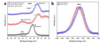
Fig. 5 High-resolution (a) Ge3d and (b) Mg1s XPS spectra of the MIMP-synthesised Mg<sub>2</sub>Ge powders with an irradiation time of 60 s.
