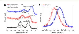
Fig. 2 High-resolution (a) Si2p and (b) Mg1s XPS spectra of MIMP-synthesised Mg<sub>2</sub>Si powders (irradiated for 60 s).
