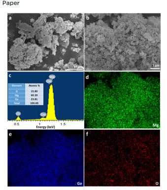
Fig. 4 SEM characterisation of Mg<sub>2</sub>Ge powders synthesised from Mg and Ge at 200 W with an irradiation time of 60 s, showing: (a and b) SEM images at different magnification: (c) a representative EDX spectrum taken from the area shown in the image in (b): and (d-f) elemental maps of Mg, Ge and O, respectively, taken from the same area shown in (b).
