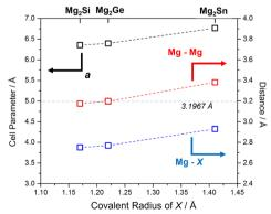
Fig. 6 Plot of refined lattice parameter, a (black), Mg-X (blue) and Mg-Mg (red) distances<sup>5</sup> for MIMP-synthesised Mg<sub>2</sub>X (X = Si, Ge, Sn) (200 W, 1 min) against covalent radius of X.60 The horizontal line and value represents the Mg-Mg distance in Mg metal. 40
