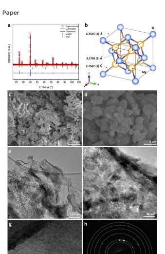
Fig. 1 Results from PXRD and electron microscopy for the MIMP-synthesised  $Mg_2Si$  powders, showing (a and b) profile plot of the Rietveld refinement against PXD data and the corresponding crystal structure; (c and d) SEM images, (e–g) TEM images, and (h) SAED pattern taken from the area shown by the image in (g).
