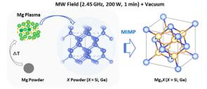
Scheme 1 Schematic of the principal Mg plasma-enabled reaction route proposed for the MIMP synthesis of Mg<sub>2</sub>Si and Mg<sub>2</sub>Ge.
