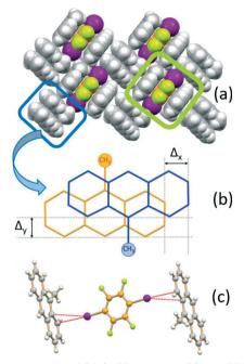
Fig. 3 Packing features of (MA)<sub>4</sub>·I2F4 showing (a) the I2F4 molecules "sandwiched" between MA molecules (lime rectangle) and the  $\pi$ -stacked MA pairs (blue rectangle), (b) details of the head-to-tail pair arrangement ( $\Delta y$  and  $\Delta x$  indicate the transversal and longitudinal offsets, respectively), and (c) the geometry of the  $I \cdots \pi$  interactions.
