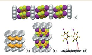
Fig. 1 (a) Space-filling representation of crystalline A·(I2F4)<sub>2</sub> showing the ladder-like alternation of anthracene and I2F4 molecules. Comparison of the layered structures in (b) solid anthracene (CSD refcode: ANTCEN) and (c) A·(I2F4)<sub>2</sub>, and (d) a depiction of the  $X \cdots \pi$ interactions at work between iodine atoms and the anthracene aromatic rings.
