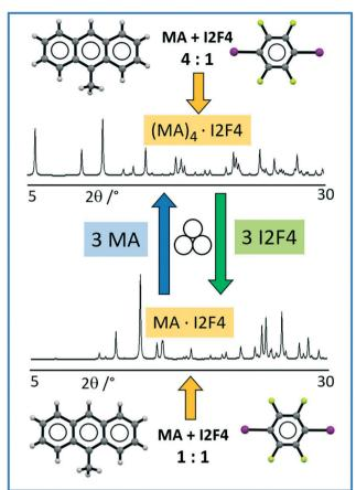
Scheme 1 Representation of mechanochemical synthesis and interconversion of crystalline (MA)<sub>4</sub>·I2F4 (top) and MA·I2F4 (bottom).
