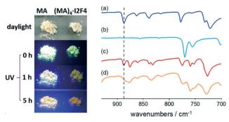
Fig. 4 Left: pictures taken during the UV irradiation of the polycrystalline samples of MA and (MA)<sub>4</sub>·I2F4. Right: details of the FTIR spectra recorded on (a) crystalline MA, (b) the head-to-tail MA photodimer, (c) co-crystal (MA)<sub>4</sub>·12F4, and (d) the resulting amorphous solid after UV irradiation (right).
