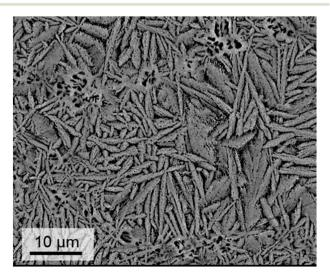
Fig. 19 Microstructure of a sinter crystallized sample with the composition 8 BaO·8 SrO·35 ZnO·45 SiO<sub>2</sub>·1 ZrO<sub>2</sub>·1 La<sub>2</sub>O<sub>3</sub>·2 B<sub>2</sub>O<sub>3</sub> sintered at 800  $^{\circ}$ C for 1 h. Redrawn from ref. 45.
