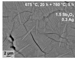
Fig. 16 SEM micrographs of glasses from the system BaO-SrO-ZnO-SiO<sub>2</sub> nucleated with Ag + Sb<sub>2</sub>O<sub>3</sub> in different concentrations after a two-step thermal treatment. Both micrographs show the same magnification.
