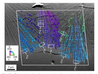
Fig. 14 Orientation of surface crystals with growing direction from the top to the bottom. The micrograph shows a cross section after crystallization for 1.5 h at 790 °C. The colour coded part of the micrograph is a superposition with an inverse pole figure map of an EBSD scan. (redrawn from ref. 50).
