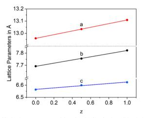
Fig. 11 Lattice parameters of  $Ba_{0.5}Sr_{0.5}Zn_2Si_{2-z}Ge_zO_7$  solid solutions with  $z=0,\,0.5$  and 1.
