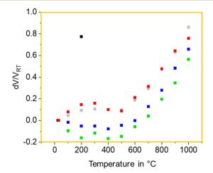
Fig. 7 Thermal expansion of  $Ba_{1-x}Sr_xZn_2Si_2O_7$  as a function of the temperature for various x-values.
