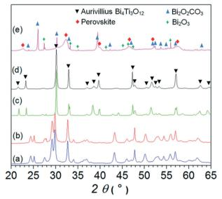
Fig. 2 XRD patterns of samples synthesized with hydrothermal treatment for 38 h at 200 °C in NaOH with different concentrations: (a)  $0.1 \text{ mol } L^{-1} \text{ NaOH, (b) } 0.5 \text{ mol } L^{-1} \text{ NaOH, (c) } 1 \text{ mol } L^{-1} \text{ NaOH, (d) } 2$ mol  $L^{-1}$  NaOH, and (e) 12 mol  $L^{-1}$  NaOH.
