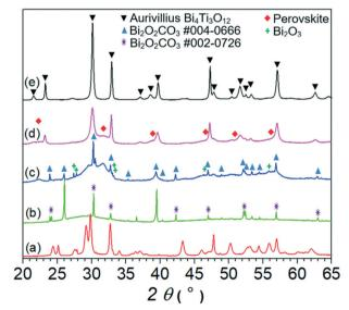
Fig. 3 XRD patterns of nanowires hydrothermally synthesized with treatment for 38 h at 200 °C in 0.5 mol L<sup>-1</sup> NaOH (a) and samples treated for different times at 200 °C in 2 mol L<sup>-1</sup> NaOH: 10 minutes (b), 1 hour (c), 3 hours (d), and 38 hours (e).
