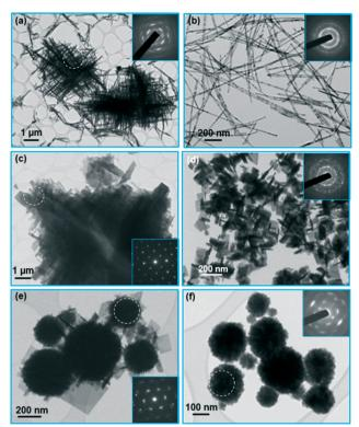
Fig. 1 TEM images with corresponding electron-diffraction patterns (the area where the pattern was recorded is marked with a white circle) of the product synthesized by hydrothermal treatment of precipitated Ti<sup>4+</sup> and Bi<sup>3+</sup> ions for 38 hours at 200 °C in NaOH of increasing concentration: (a) 0.1 mol  $L^{-1}$ , (b) 0.5 mol  $L^{-1}$ , (c) 1 mol  $L^{-1}$ , (d) 2 mol  $L^{-1}$ , (e) 8 mol  $L^{-1}$ , and (f) 12 mol  $L^{-1}$ .
