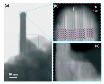
Fig. 5 BF (a) and HAADF ((b) and (c)) STEM images of the bismuthtitanate nanoplatelet growing on the surface of the nanoparticle aggregate. (a) and (b) The model of the Aurivillius structure projected along the [110]<sub>AU</sub> direction is superimposed over the image (b) to illustrate the positions of the Bi<sup>2+</sup> and Ti<sup>4+</sup> ions. Double magenta lines in Fig. 5(c) show the position of the  $(Bi_2O_2)^{2+}$  structural layers.
