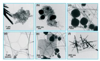
Fig. 7 Product nanoparticles after hydrothermal treatment for different times at 200 °C in KOH: (a) 10 minutes in 2 mol  $L^{-1}$  KOH, (b) 1 hour in 2 mol  $L^{-1}$  KOH, (c) and (d) 38 hours in 2 mol  $L^{-1}$  KOH, (e) 3 days in 2 mol  $L^{-1}$  KOH, and (f) 38 hours in 0.5 mol  $L^{-1}$  KOH.
