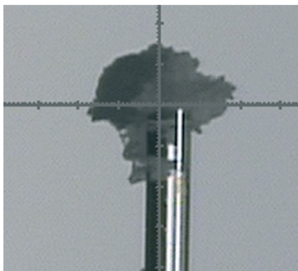
Fig. 1 A very small amount of powder (ca. 0.01 mg) mounted on the top of a glass fibre in the single crystal X-ray diffractometer. Each major tick represents 0.1 mm.
