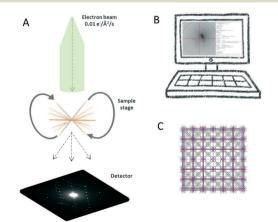
Fig. 2 Workflow of continuous rotation methods for 3D ED. (A) A fast camera records the diffraction patterns over a desired exposure time while the sample stage is continuously rotated under the electron beam. (B) The raw image data are processed to extract the intensities. (C) Structures of nanometer-sized crystals are solved *ab initio*.
